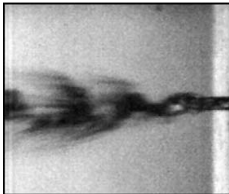
FIGURE 10. Instantaneous initial breakup image, D_l = 0.32 mm, U_g = 165 m s -1 , U_l = 16.5 m s -1 , We = 116 , Re_g = 1.1 \times 10^5 , Re_l = 5280 , m = 0.07 , M = 0.12 .
