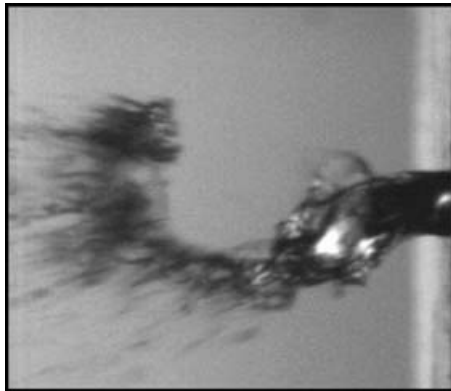
FIGURE 5. Instantaneous initial breakup image, D_l = 1.0 mm, U_g = 69 m s -1 , U_l = 1.7 m s -1 , We = 74 , Re_g = 4.6 \times 10^4 , Re_l = 1700 , m = 0.17 , M = 1.9 .
